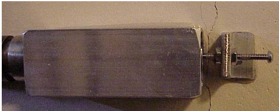
Figure 2.8 LVDT Mounting Bracket
